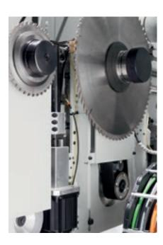
The motorised vertical blade adjustment ensures precise, quick adjustment of blade protrusion.
